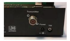
The back panel has SO-239s for connecting UHF type connectors to the antenna and transmitter. A coaxial power jack with center positive is used to provide DC power to the tuner. The jack mates with a 5.5 OD, 2.5 ID coaxial power plug. Between 11 and 15 volts DC can be used. The power supply must be able to provide up to 0.5 amps.
