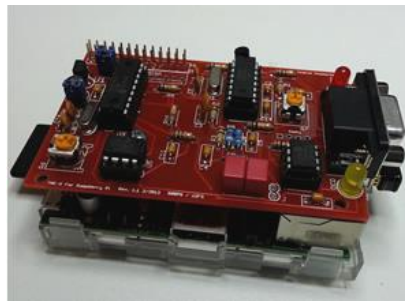
Figure 2: TNC-Pi mounted on a Raspberry Pi
